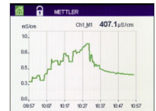
Historic data can be displayed as a trend measurement with one second updates.
